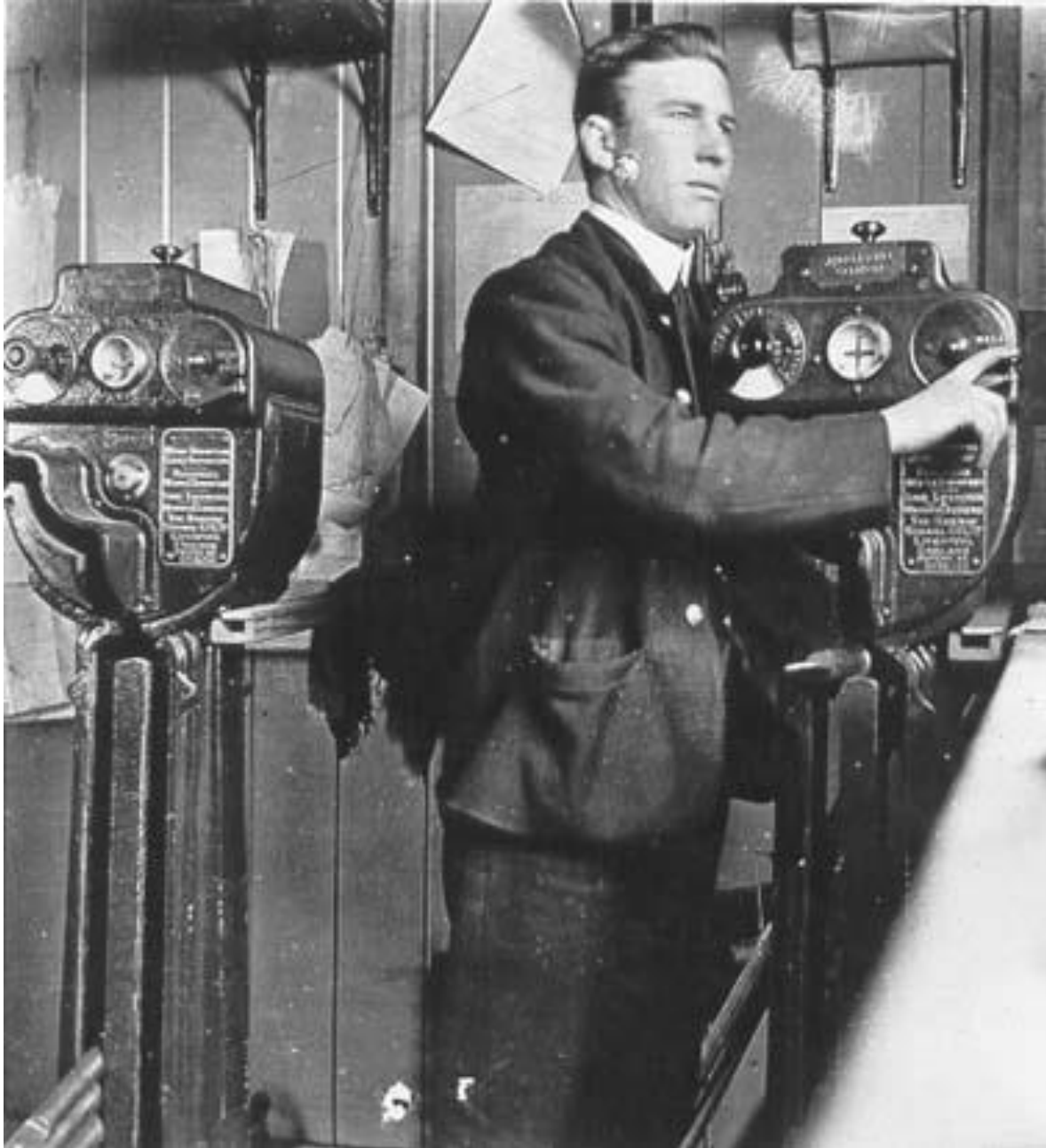
Signalman tapping out a bell code on a Staff Instrument at an unknown location.
