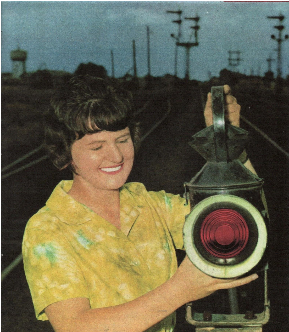
Assistant Gatekeeper Carmel Scanlon, pictured is shown above placing a kerosene lit gate lamp on one of the hand gates at Horsham. It appeared in the April 1966 Issue of the then Victorian Railways Newsletter. Hand operated gates have now long disappeared from the railway scene and the picture in that sense is now quite historic.
