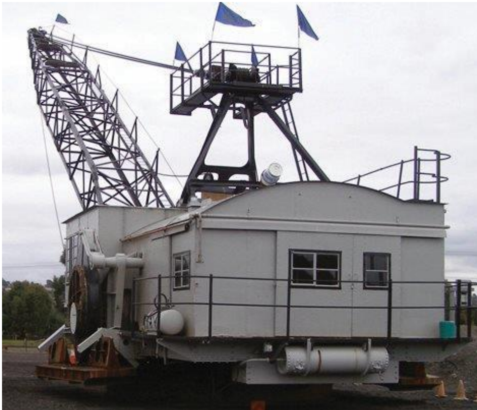
Pic 2 - Rapier walking Dragline
