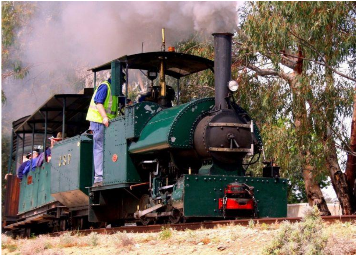
Bagnall 0-4-0 ST Loco and passenger train hard at work on the 2'00" gauge tramway.
