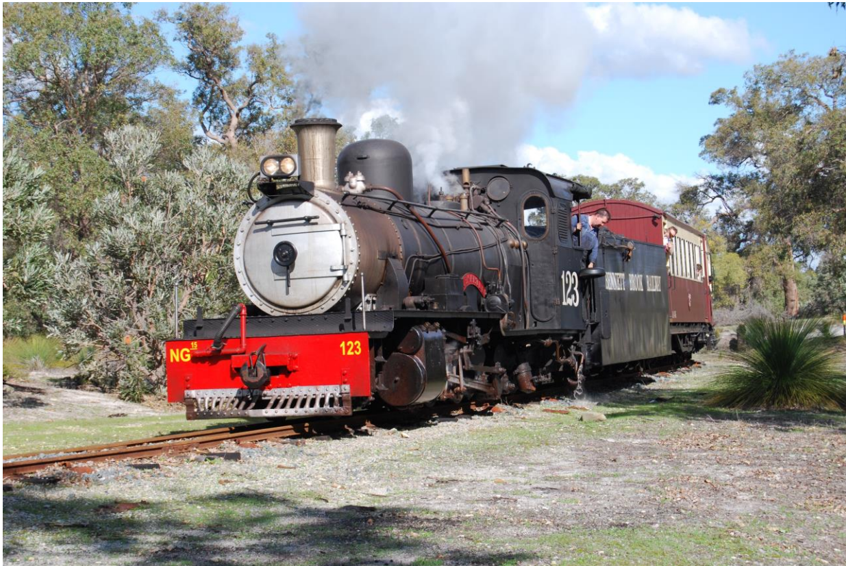
NG15-123 2-8-2 Steam Loco and Passenger train running along the Bennett Brook Railway.
