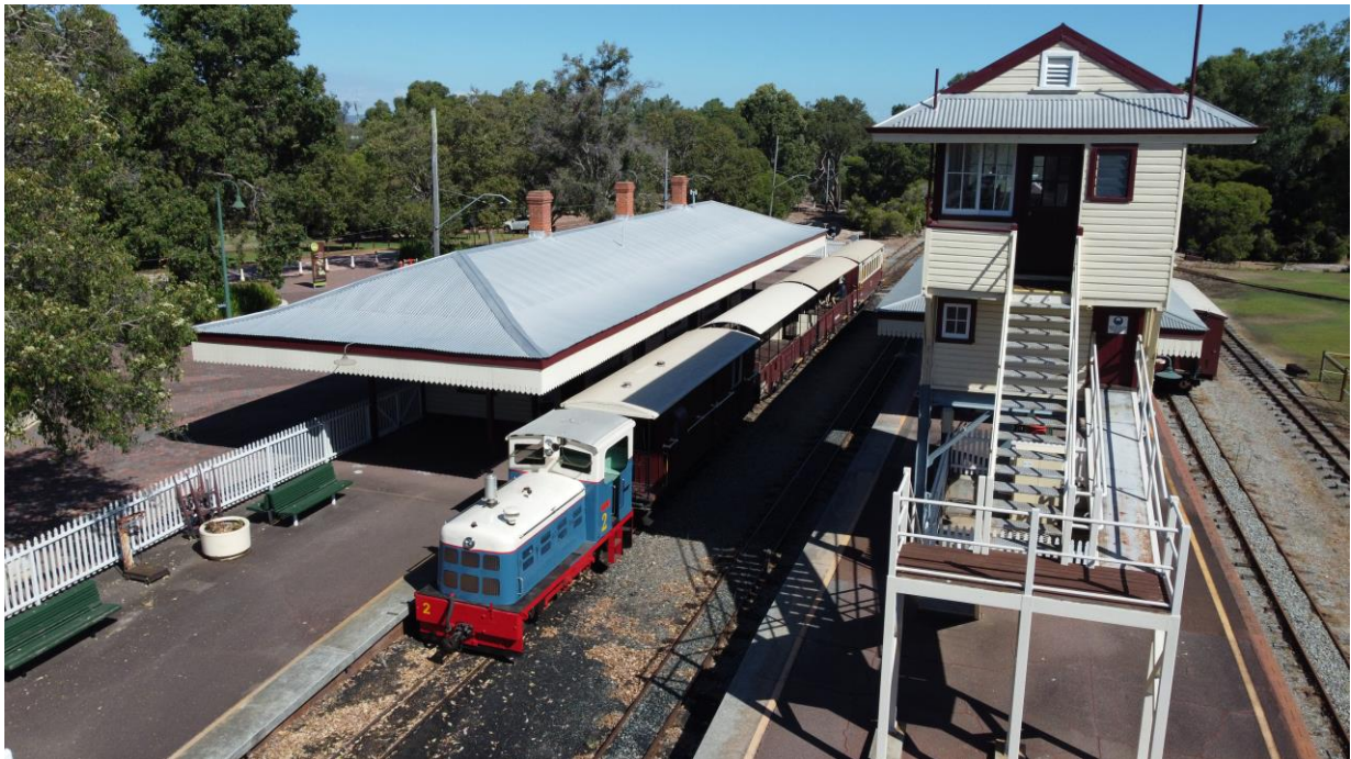
Fowler No.2 0-6-0 DH Loco and Passenger train await departure time at Whiteman Village Junction. The elevated Signal Box (which was originally at Subiaco) controls the stations comings and goings with a 40 lever Interlocked Signal Frame.
