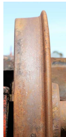
Above: New tyres at Newport Workshops. Right: a wheel on a YVR bogie showing showing a worn profile
